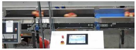
The Separation Unit optimises the distance between the bags, which helps to increase the speed of the line.
